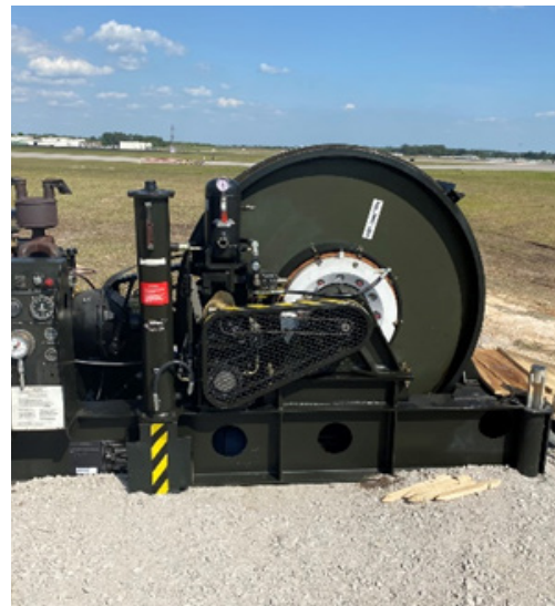
Temporary Bak-12 arrestor cable
